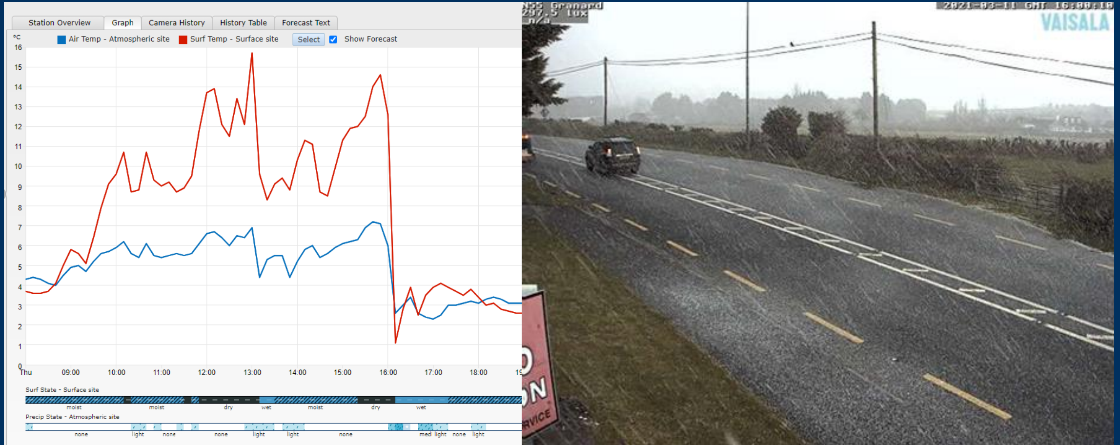
Road Surface Temperature Profile in Red (Air Temp in Blue) showing a 14°C drop around 1600 during a hail shower on March 11 th at Granard, County Longford
